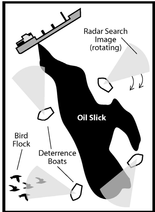
**Fig. 2.** A radar-activated on-demand system would require multiple ships to cover a large spill effectively and to continue moving with the drifting slick.
