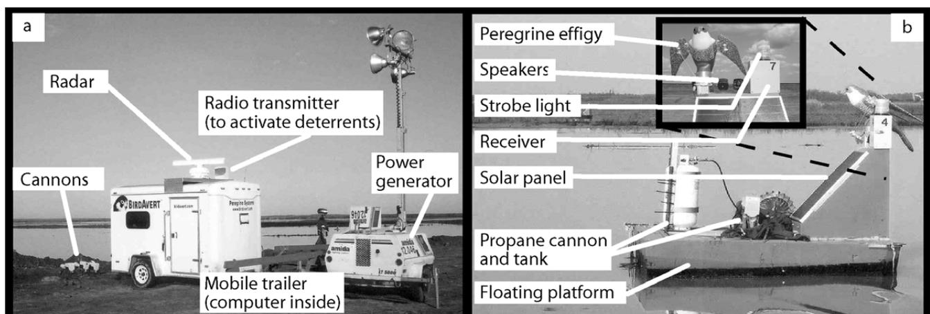
Fig. 1. The BirdAvert (Peregrine Systems, Salt Lake City, Utah, USA) on-demand radar-activated system.
