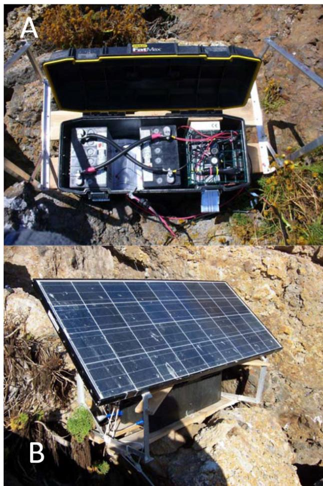
**Fig. 6:** Vocalization broadcast system on Orizaba Rock, 2011: (A) tote box containing MP3 player and other equipment and (B) close-up of solar panel and tote box (photos by L. Harvey).
