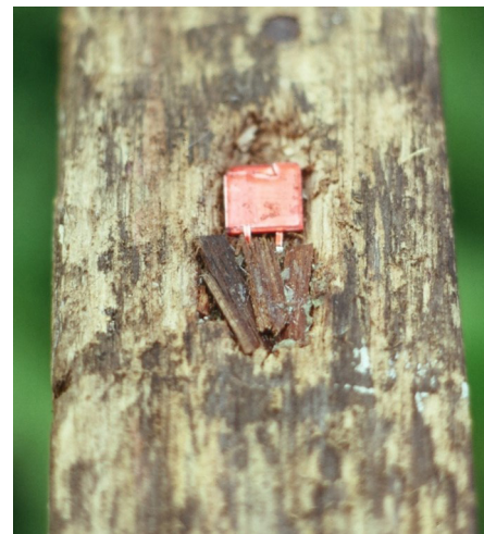
Fig. 2. View from above of piezo-electric microphone that was placed on top of the wooden T-piece where one of the White Terns Gygis alba incubated its egg. Wood chips embedded in paste protect the leads to the microphone from damage by the bird's feet.
